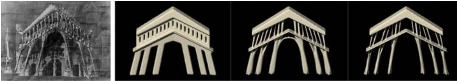
**Figure 1 Passion Façade Figure 2-4 Passion Façade ESO model
