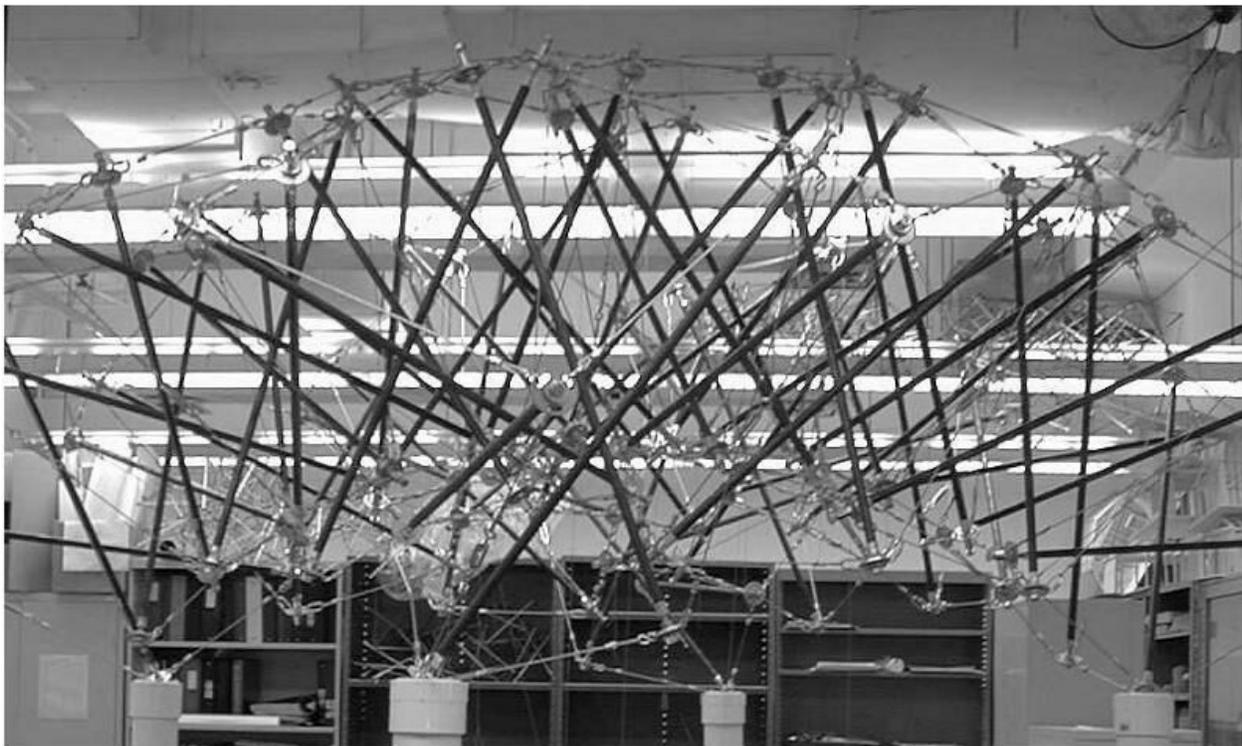
Figure 15. Model of a tensegrity dome composed by sixteen units of square base
